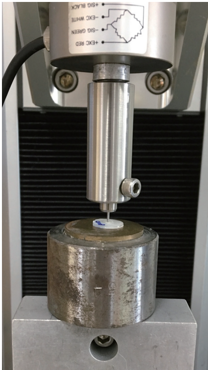
Fig. 1. A cylindrical stainless steel plunger of the universal testing machine on calcium silicate-based biocompatible material inside a lumen of a root section specimen.
