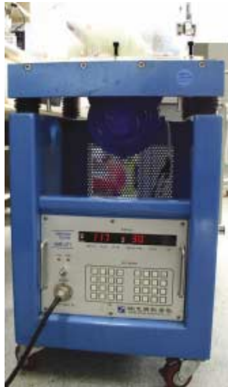
Fig. 1. Mechanical vibration machine was used to stimulate whole body vibration for rats.
