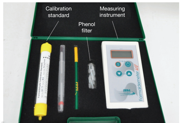
Fig. 3. Measuring instrument for formaldehyde concentration.
