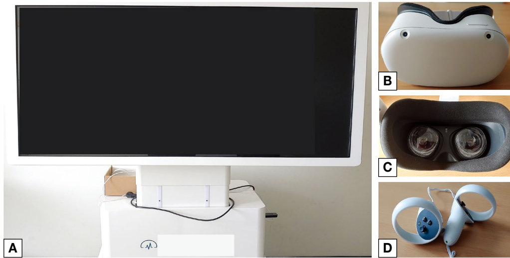
Fig. 1. MDBOX VR consists of a hardware with monitor (A), head-mount display (B and C), and joystick (D).
