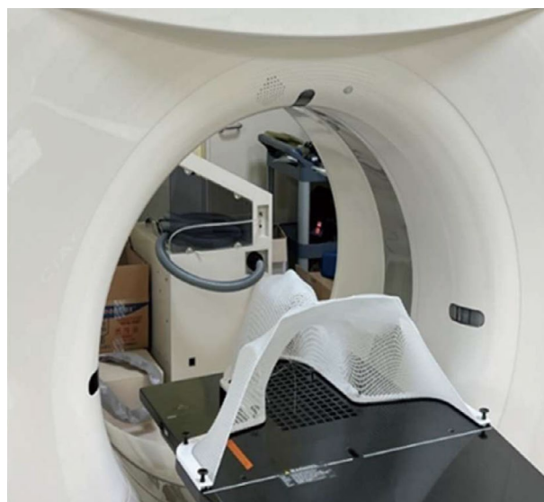
Fig. 3. CT acquisition setup for three-dimensional evaluation of thermoplastic head-and-neck mask deformation after molding.
