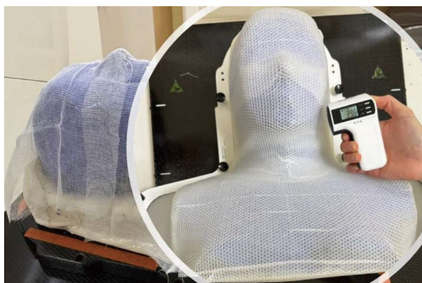
Fig. 2. Locations of temperature measurement points on the thermoplastic head-and-neck mask and example of surface temperature measurement on the anthropomorphic head-and-shoulder phantom.
