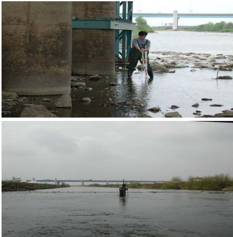
<그림 2> Scene of observed runoff by walking method
