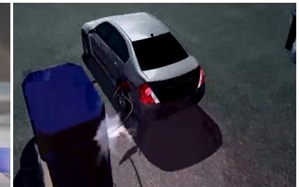
<Fig 12> The Scene Separated Hose with Lubricator Start by Departure of the Car.
