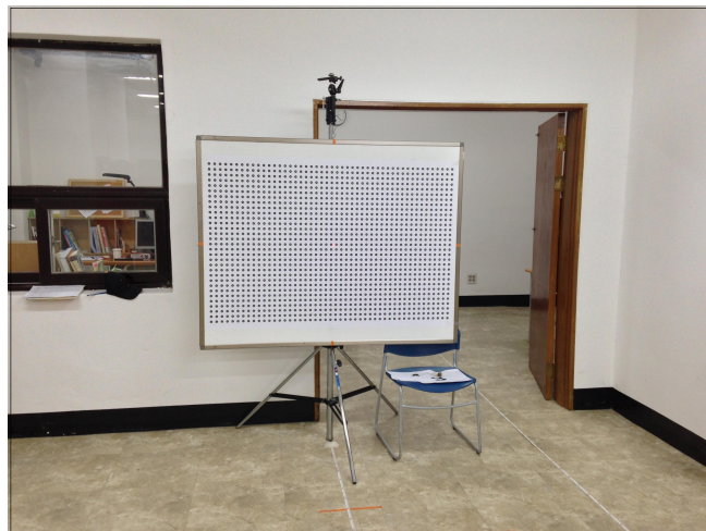
<Fig 5> Calibration Plate for Camera Calibration
