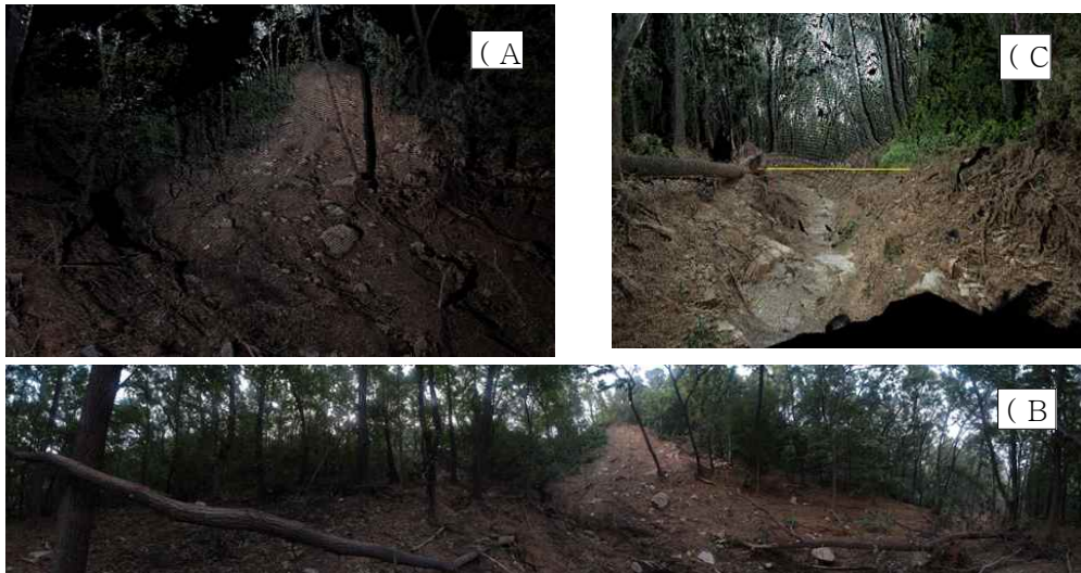
<Fig 3> Scanning of Debris Flow Track, (A) RGB Data, (B) Panorama Image Data, (C) Measurement of Bed Width
