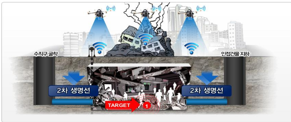
(b) Relief method using horizontal excavation (Use adjacent buildings and vertical holes)
