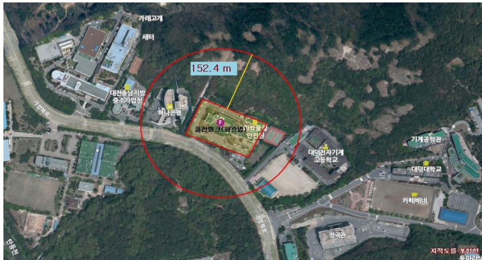
Figure 6. Diagram of ERPG-2 dispersion result for case A(1.0 m distance).
