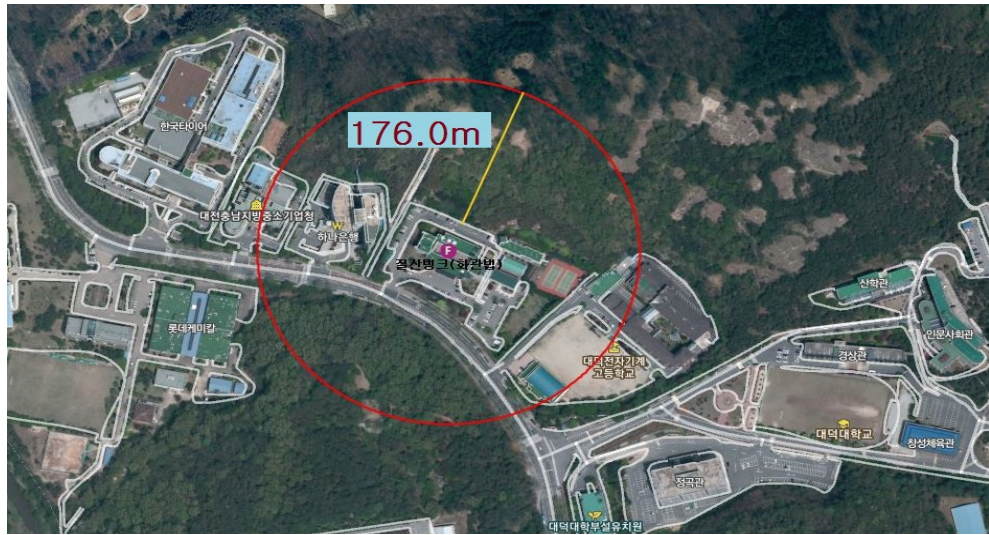
Figure 5. Diagram of ERPG-2 dispersion result for case A(1.5 m distance).
