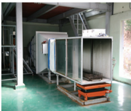
Figure 1. Wind tunnel device for measure flame spread rate
