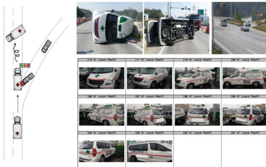
Figure 5. Accident description and pictures of damaged vehicle in case II
