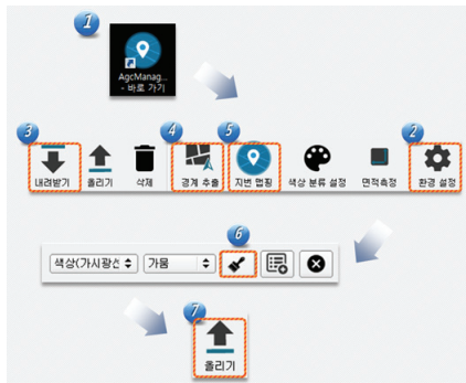
Figure 17. Steps to use automatic assessment software for rice field damage area
