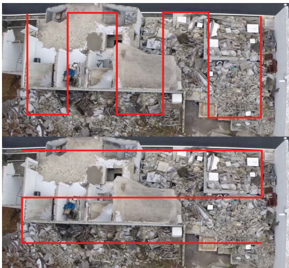
Figure 13. Image acquisition path with 50% overlapping
