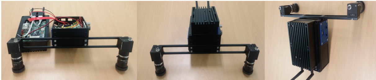
Figure 1. Manufactured stereo camera module
