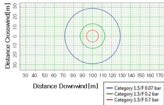
Figure 4. Distance and explosion pressure when VCE occurs (Worst case scenario, UPE Resin)
