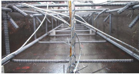
(a) Vertical thermocouples
