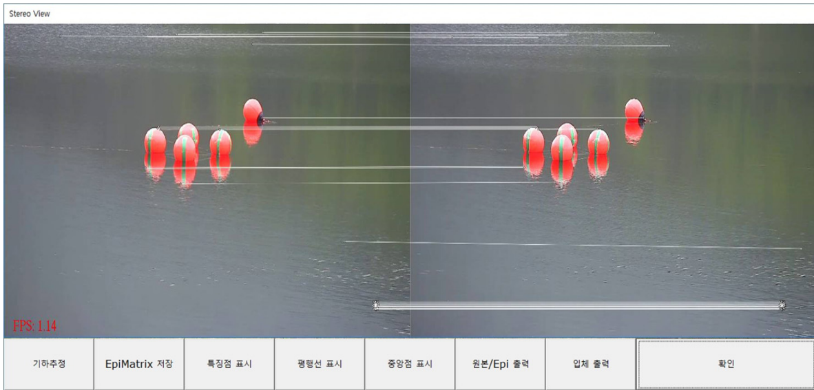
Figure 9. Keypoint extraction of left and right images
