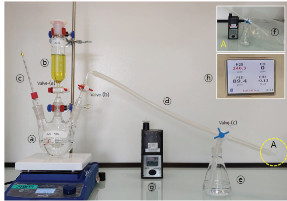
Figure 4. Schematic diagram of reaction between sodium hydrogen sulfide and sulfuric acid
