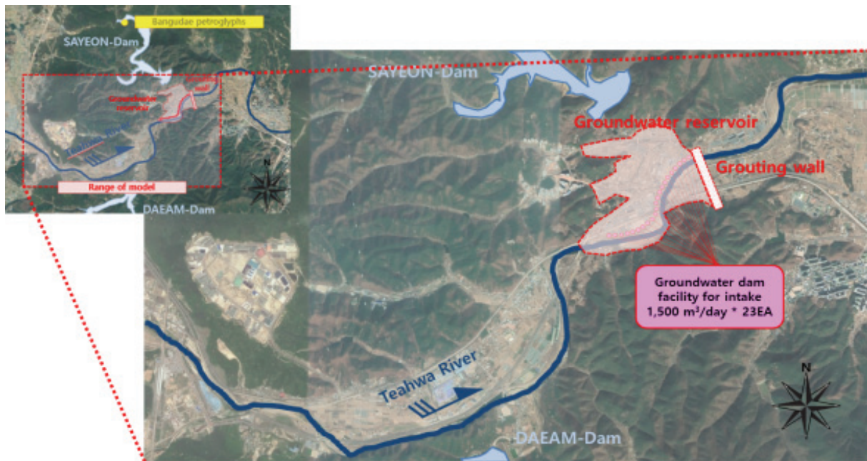
Figure 11. Apply to intake facility of groundwater reservoir
