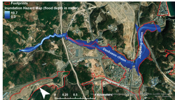
※ Source: LX(2019). for the footprints. Figure 13. Inundation hazard map and footprints for Naedeok reservoir, GiJang-gun
