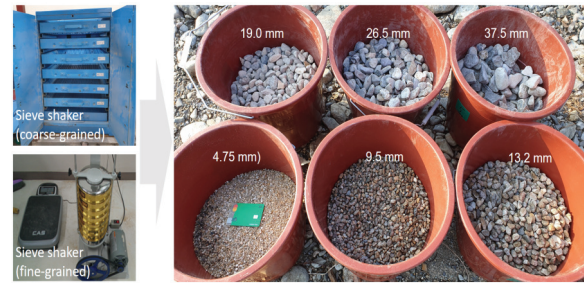
Figure 9. Classification of grain sizes using sieve shaker
