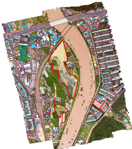
Figure 7. Orthomosaic image taken by UAV. Red poly-line means flooded area
