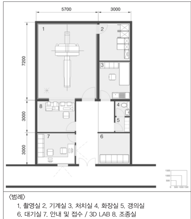
[Figure 7] Planning of the CT Unit-1 / Single Examination Room
