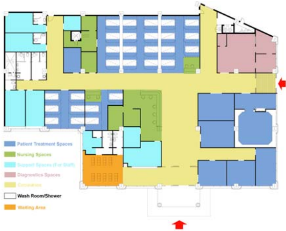
[Figure 8] Floor Plan of Emergency Medical Center of Seoul National University Bundang Hospital
