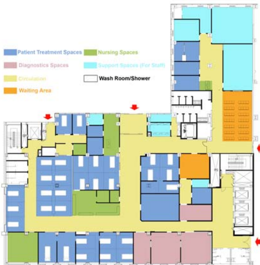
[Figure 4] Floor plan of emergency Medical Center Gachon University Gil Medical Center
