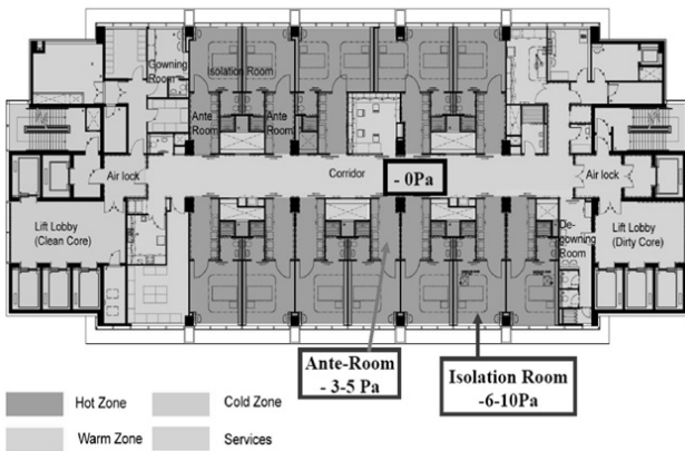
[Figure 1] Typical Floor Plan of PMH Isolation Unit source : Owen Tsang' ppt, Hospital Authority, Hongkong, 2015
