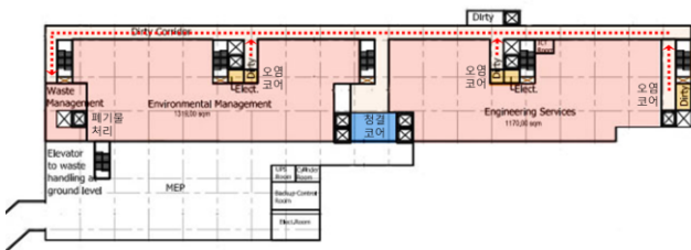
[Figure 16] Waste and Environment Service Floor Plan(Basement 1st) of Kuwait Infectious Diseases Hospital
