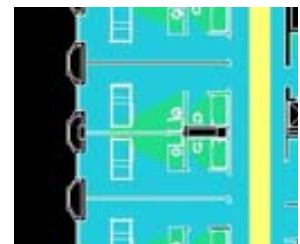
2-2. Low Visibility. The patient in room is visible only from corridors. The light blue area indicates the one that is visible from the corridor. Most patients in rooms were visible from the corridor.
