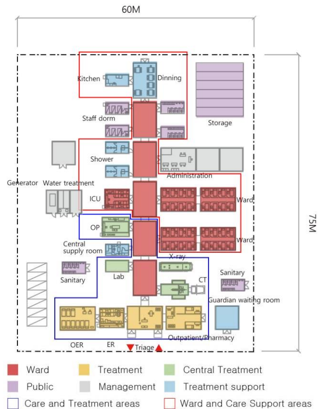
[Figure 7] 'P' Company Mobile Hospital Alt 3 Function and Area Analysis Diagram in 2017
