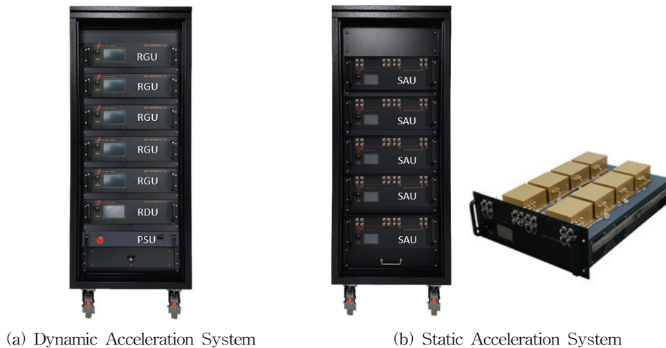
<Figure 11> Semiconductor RF lifetime evaluation system including dynamic and static acceleration
