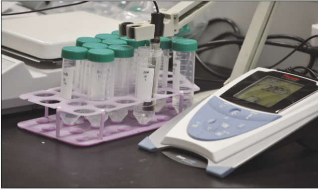
Fig. 3. Fluoride sensitive electrode (Orion 9609, Thermo Scientific, USA) and pH/ISE meter (Orion 4 star, Thermo Scientific, USA) were used in the study.
