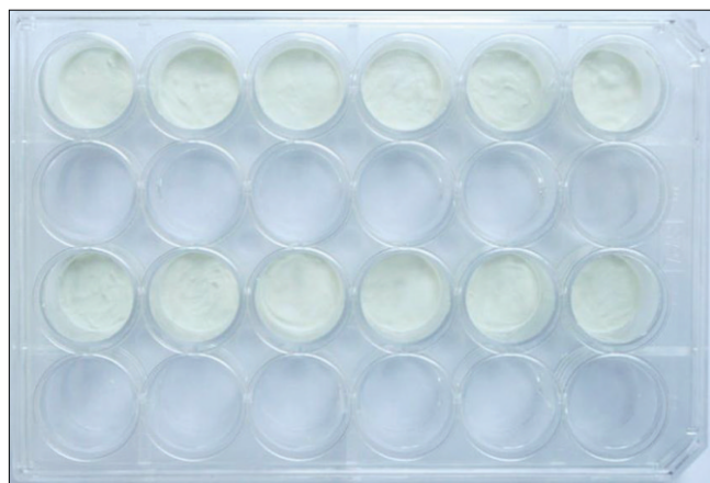
Fig. 1. White MTA coated onto 24-well culture plates. The first and third rows are coated with white MTA while the second and fourth rows are left uncoated for the control.
