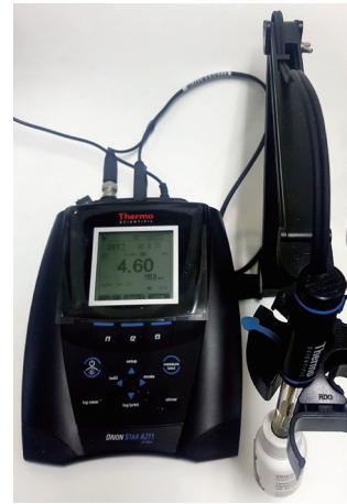
Fig. 3. pH meter used to measure pH over time in this study.
