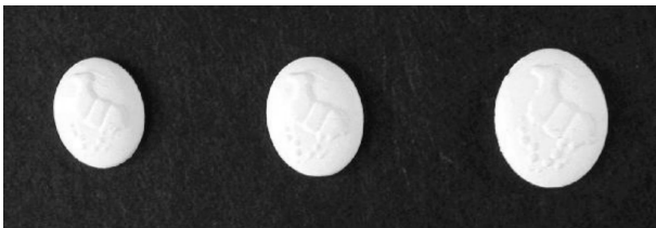
Fig. 1. Photograph of pearl nucleus obtained using the mold with goral shape.
