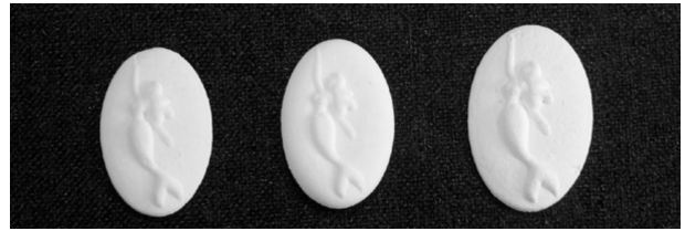
Fig. 3. Photograph of pearl nucleus obtained using the mold with mermaid shape.
