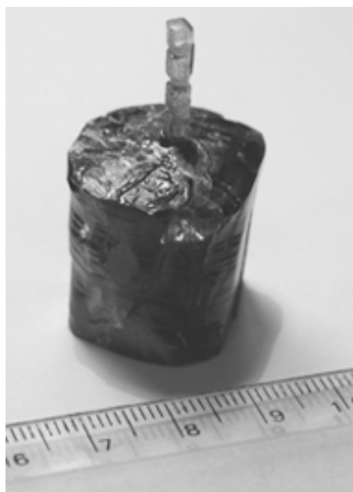
Fig. 2. As-grown 1 inch \text{LuVO}_4 single crystal.
