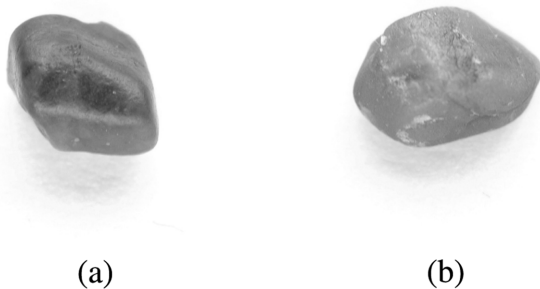
Fig. 1. Photographs of Australian natural sapphire (a) non-treated and (b) hydrothermally treated at 350°C for 3 days in 2 M NaOH solution.
