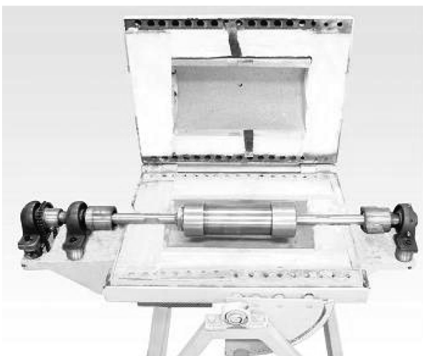
Fig. 1. Photograph of apparatus used for hydrothermal synthesis of mica.
