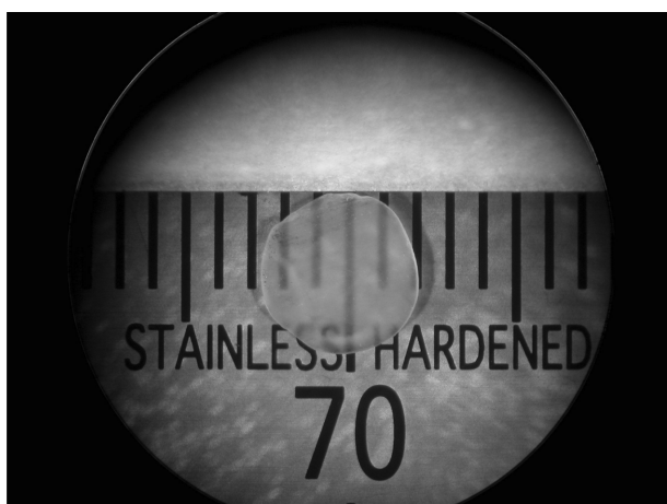
Fig. 3. Sliced and polished specimen of \text{MgAl}_2\text{O}_4/\text{MgO} eutectic.
