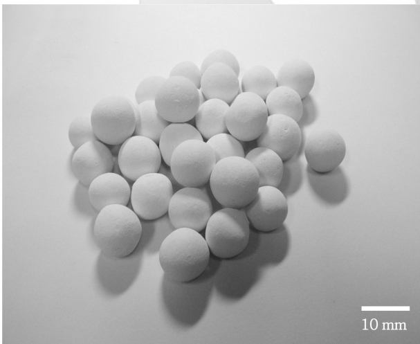
Fig. 5. Photograph of the porous ceramic balls impregnated with Ag colloid.
