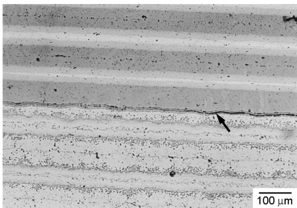
Fig. 3. Optical micrograph of composite fabricated from Ni/Al.../Ti/Al stacked foils, using hot pressing process.
