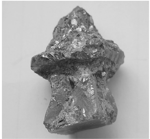
Fig. 5. PZN-PT crystal grown by the two-step process.
