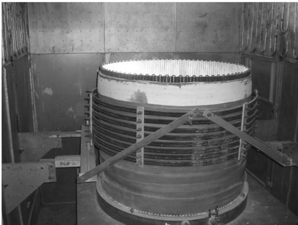
Fig. 1. Photograph of skull melting apparatus.
