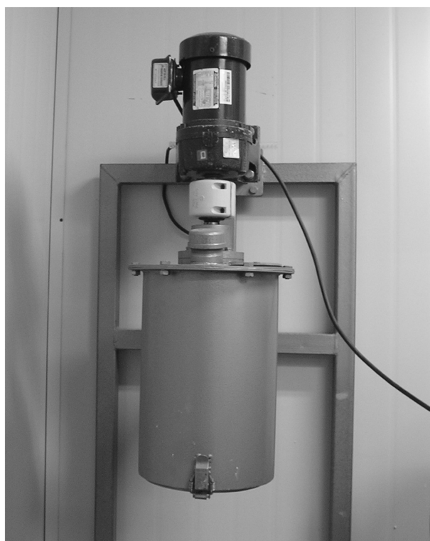
Fig. 3. Photograph of the stirrer used for surface coating of synthetic mica
