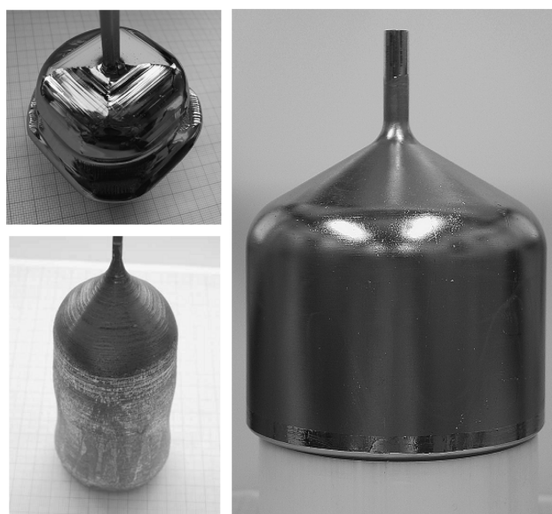
Fig. 5. GaAs (a, b) and Ge (c) single crystals grown by VCz (a), LEC (b) and VGF (c) under TMF generated in combined heater-magnet modules.
