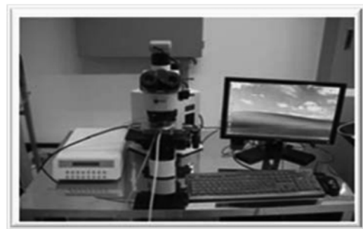
Fig. 2. A furnace system with the in-situ microscope for sample annealing.
