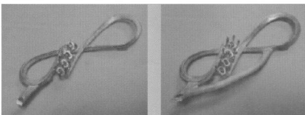
Fig. 15. Feed sprue single, double.
