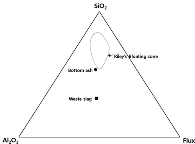
Fig. 2. Ternary diagram of ceramic composition. The area surrounded by dotted line represents the bloating zones during sintering process presented by Riley [7].
