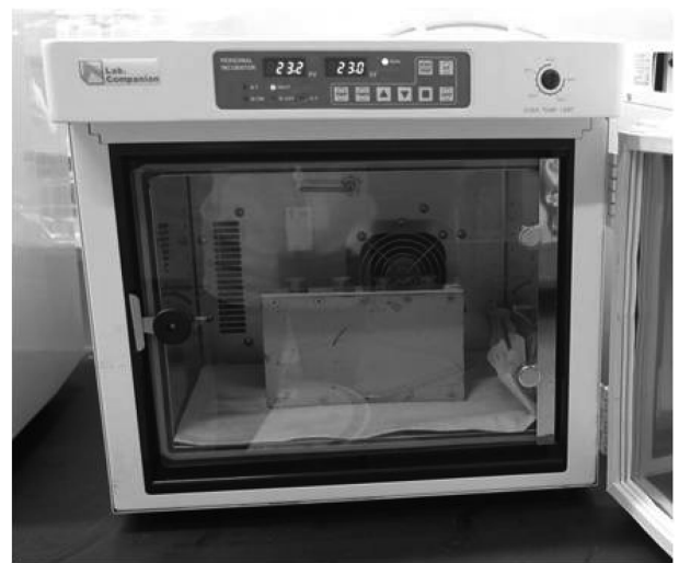
Fig. 9. The magnetic device with the tubes is placed into an incubator.
