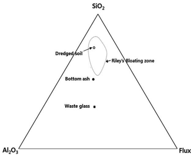
Fig. 1. Ternary diagram of ceramic composition showing the bloating zones during sintering process presented by Riley [11]. The specimens fabricated in this study are included in the Riley's bloating zone (●: bottom ash, ○: dredged soil, ■: waste glass).
