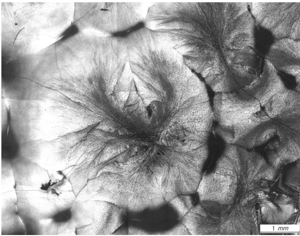
Fig. 7. Optical micrograph of diopside crystal ( \times 50 ).
